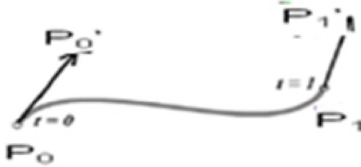
Figure 4: Hermite Specification Control points P_0, P_1 and Slopes P'_0, P'_1 .
